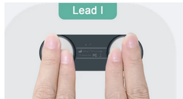
Figure 1. Most gadgets can record lead I, e.g., by touching the two electrodes with the finger(s) of each hand
