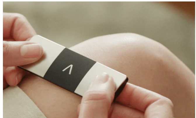
Figure 5. KardiaMobile 6L records a 6-lead ECG with 2 sensors on top and 1 sensor on the bottom ( Error! Hyperlink reference not valid. )
